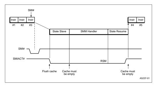
Figure 8-1. Basic SMI# Interrupt Service
