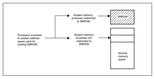
Figure 8-5. Redirecting System Memory Addresses to SMRAM
