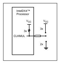
Figure 9-3. Voltage Detect (VOLDET) Sense Pin
