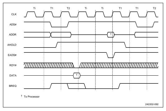
Figure 10-26. Typical Internal Cache Invalidation Cycle
