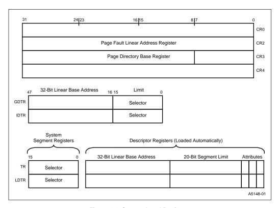
Figure 4-4. System-Level Registers
