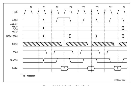
Figure 10-21. 8-Bit Bus Size Cycle
