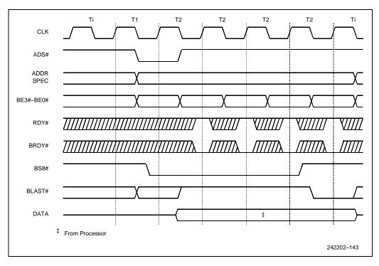
Figure 10-22. Burst Write as a Result of BS8# or BS16#
