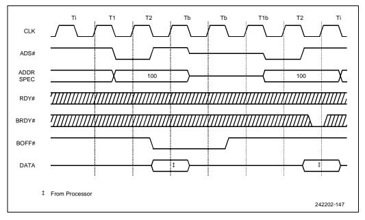
Figure 10-34. Restarted Write Cycle
