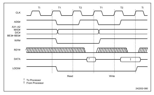
Figure 10-23. Locked Bus Cycle
