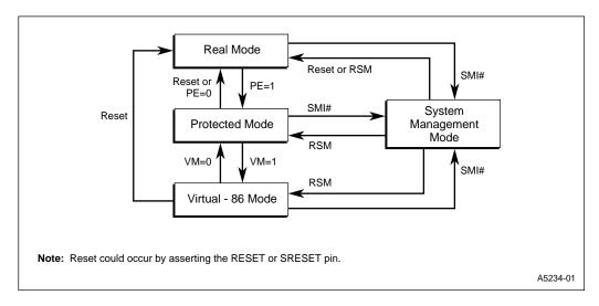
Figure 8-6. Transition to and from System Management Mode
