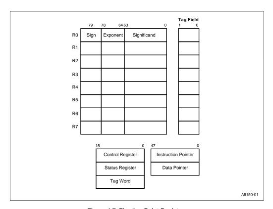
Figure 4-7. Floating-Point Registers
