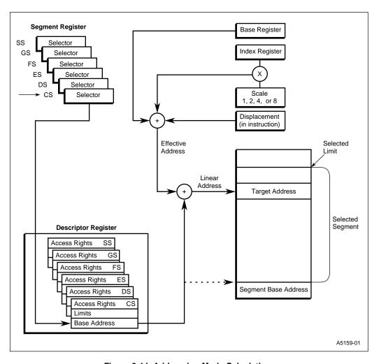
Figure 3-14. Addressing Mode Calculations
