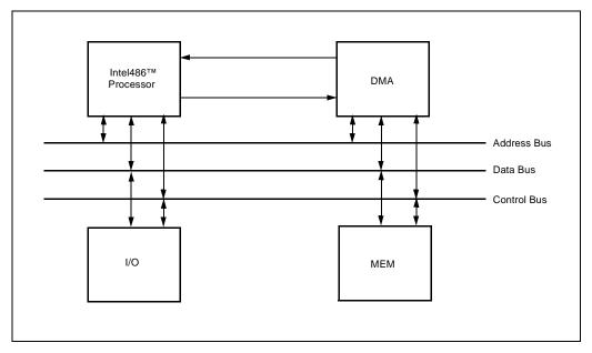
Figure 10-8. Single Intel486™ Processor with DMA
