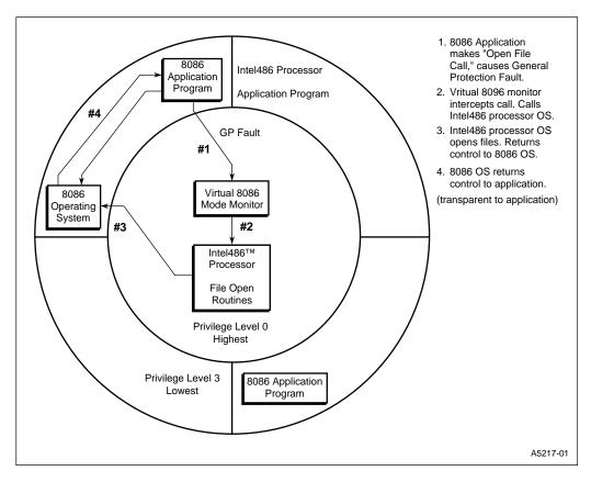
Figure 6-25. Virtual 8086 Environment Interrupt and Call Handling
