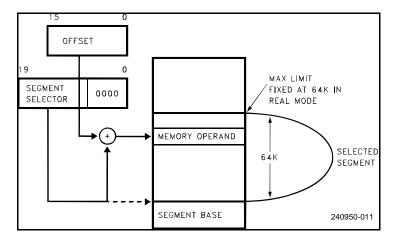
Figure 5-1. Real Address Mode Addressing
