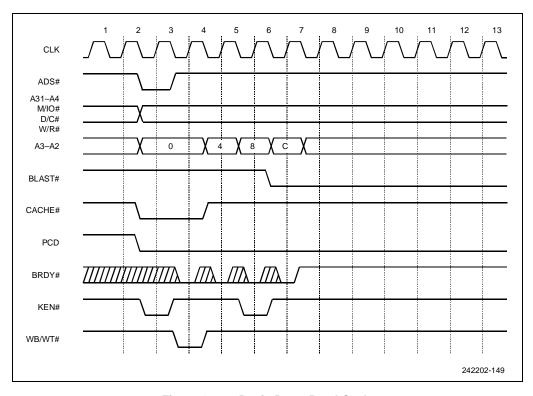
Figure 10-37. Basic Burst Read Cycle
