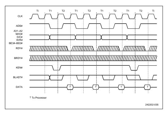
Figure 10-14. Non-Burst, Cacheable Cycles
