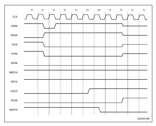
Figure 10-30. HOLD Request Acknowledged during BOFF#
