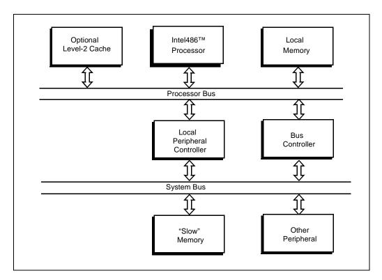
Figure 2-1. Embedded Personal Computer and Embedded Controller Example
