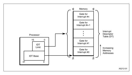
Figure 6-4. Interrupt Descriptor Table Register Use
