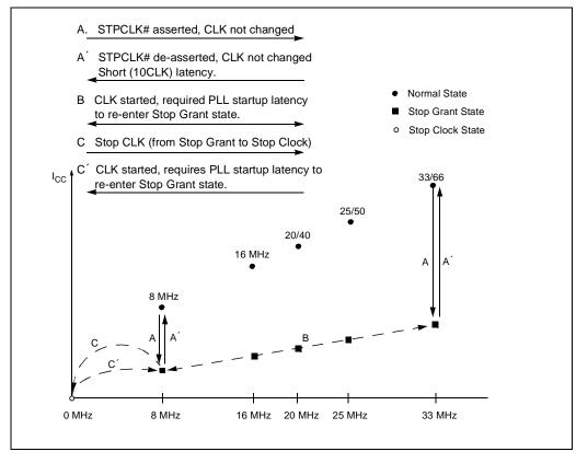
Figure 9-12. Supply Current Model for Stop Clock Modes and Transitions for the Intel486™ Processor
