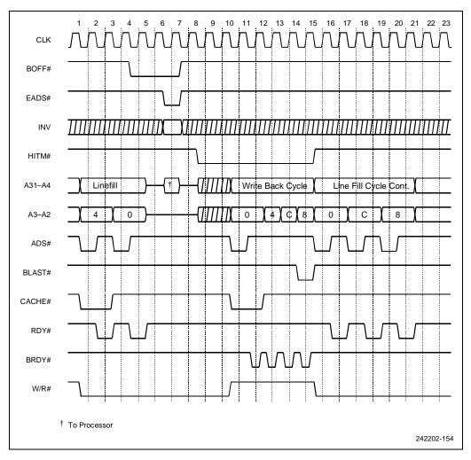
Figure 10-42. Snoop under BOFF# during a Cache Line-Fill Cycle
