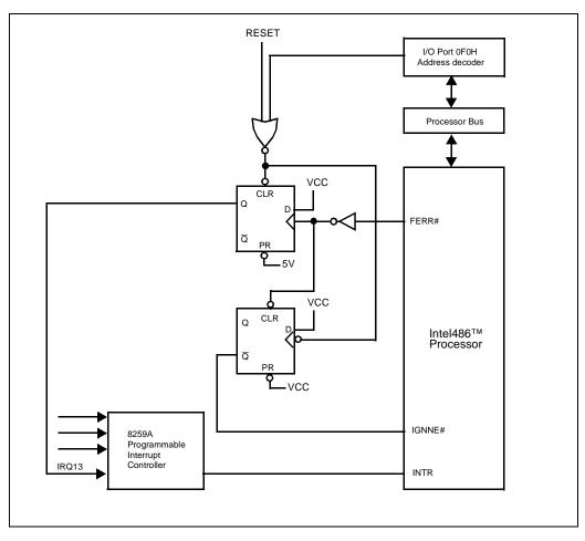
Figure 10-36. DOS-Compatible Numerics Error Circuit
