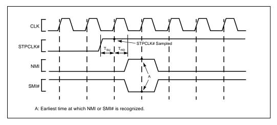
Figure 9-10. Recognition of Inputs when Exiting Stop Grant State
