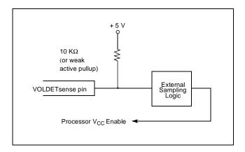
Figure 9-4. Voltage Detect (VOLDET) Sense Pin
