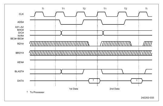
Figure 10-12. Non-Cacheable, Non-Burst, Multiple-Cycle Transfers
