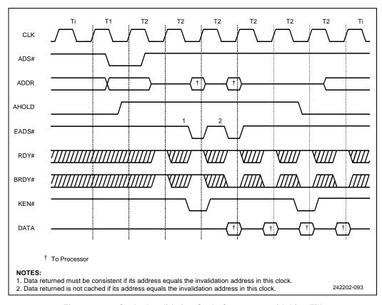
Figure 10-28. Cache Invalidation Cycle Concurrent with Line Fill
