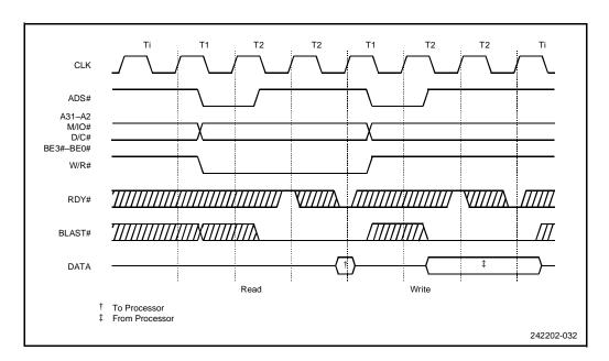
Figure 10-11. Basic 3-3 Bus Cycle
