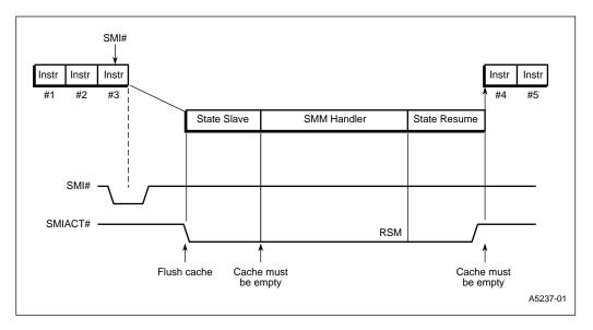
Figure 8-13. FLUSH# Mechanism during SMM
