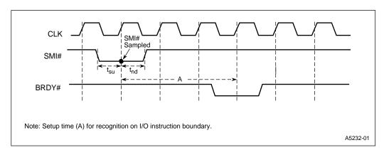
Figure 8-3. SMI# Timing for Servicing an I/O Trap
