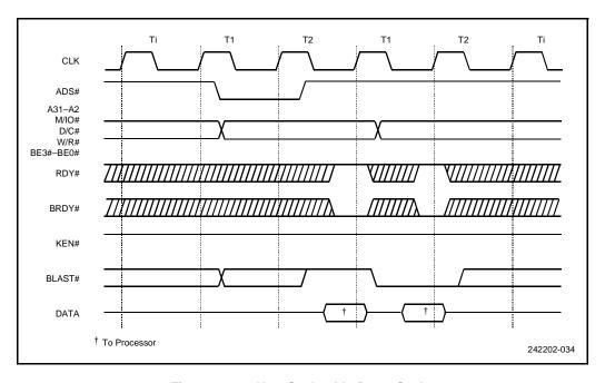
Figure 10-13. Non-Cacheable Burst Cycle
