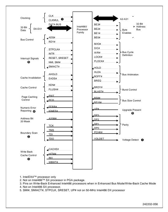
Figure 9-1. Functional Signal Groupings
