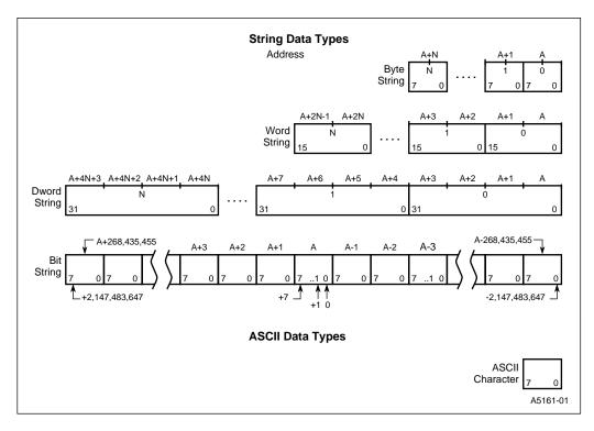
Figure 3-16. String and ASCII Data Types
