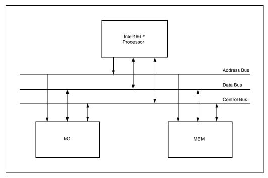
Figure 10-7. Single Master Intel486™ Processor System
