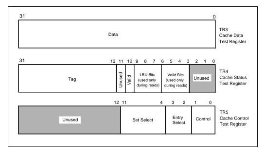
Figure B-2. IntelDX4™ Processor Cache Test Registers
