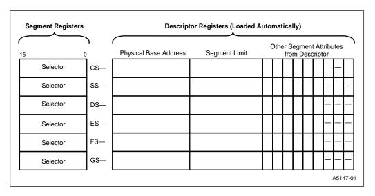
Figure 4-3. Intel486™ Processor Segment Registers and Associated Descriptor Cache Registers
