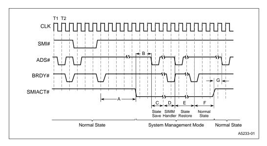
Figure 8-4. Intel486™ Processor SMIACT# Timing
