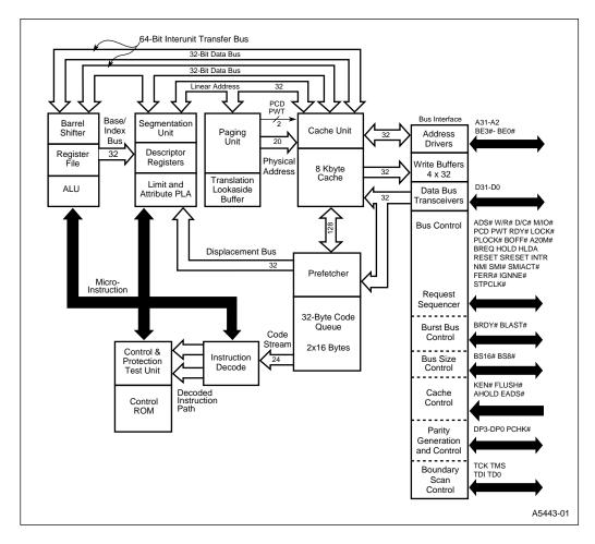
Figure 3-2. Intel486™ SX Processor Block Diagram
