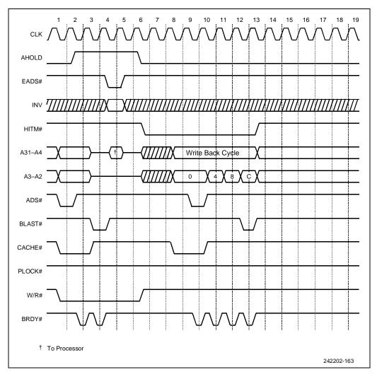
Figure 10-51. Snoop under BOFF# Overlaying a Pseudo-Locked Cycle
