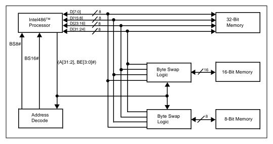
Figure 10-6. Data Bus Interface to 16- and 8-Bit Memories
