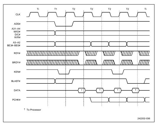
Figure 10-15. Burst Cacheable Cycle
