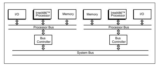
Figure 3-11. Loosely Coupled Multi-processor System
