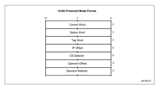
Figure 4-12. Protected Mode FPU Instruction and Data Pointer Image in Memory—16-Bit Format
