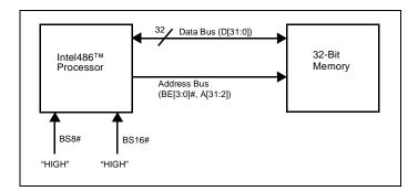
Figure 10-3. Intel486™ Processor with 32-Bit Memory
