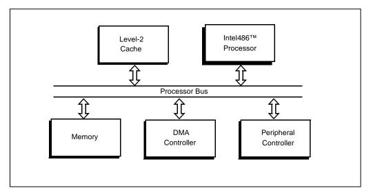
Figure 3-10. Single-Processor System
