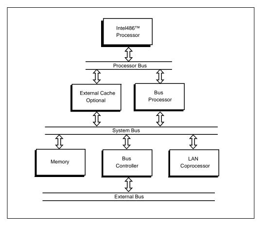
Figure 3-9. A Typical Intel486™ Processor System
