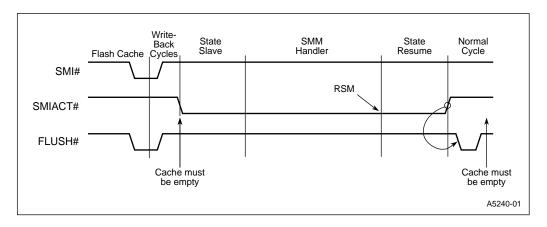
Figure 8-16. Write-Back Enhanced IntelDX4™ Processor Cache Flushing for Overlaid SMRAM upon Entry and Exit of Cached SMM
