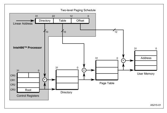
Figure 6-19. Paging Mechanism
