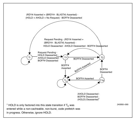
Figure 10-35. Bus State Diagram
