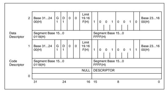
Figure 6-18. GDT Descriptors for Simple System
