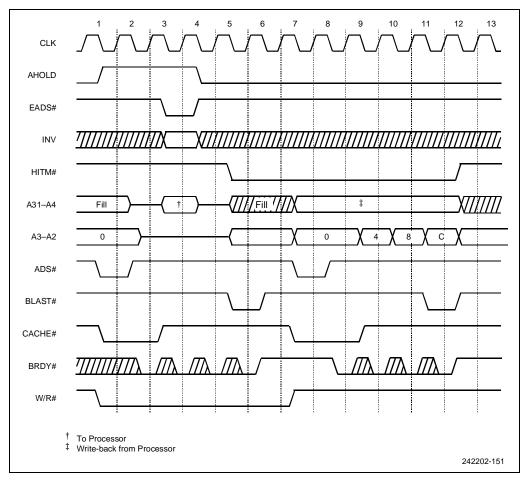
Figure 10-39. Snoop Cycle Overlaying a Line-Fill Cycle
