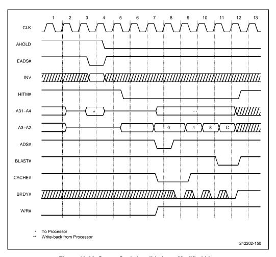
Figure 10-38. Snoop Cycle Invalidating a Modified Line
