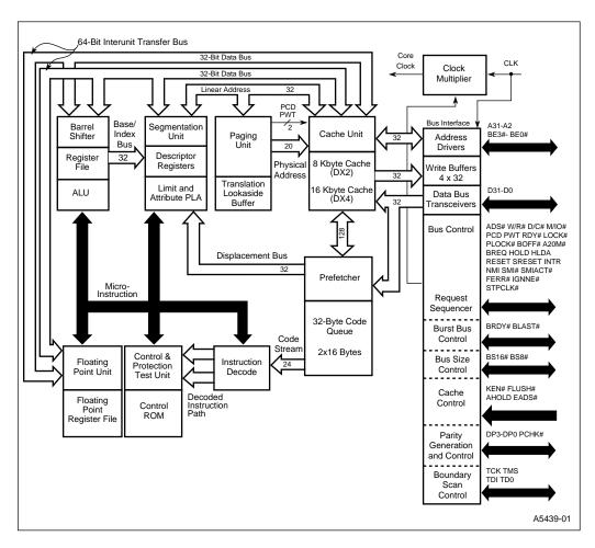
Figure 3-1. IntelDX2™ and IntelDX4™ Processors Block Diagram
