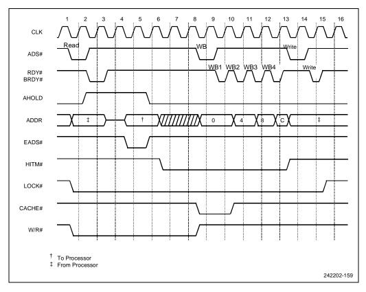
Figure 10-47. Snoop Cycle Overlaying a Locked Cycle
