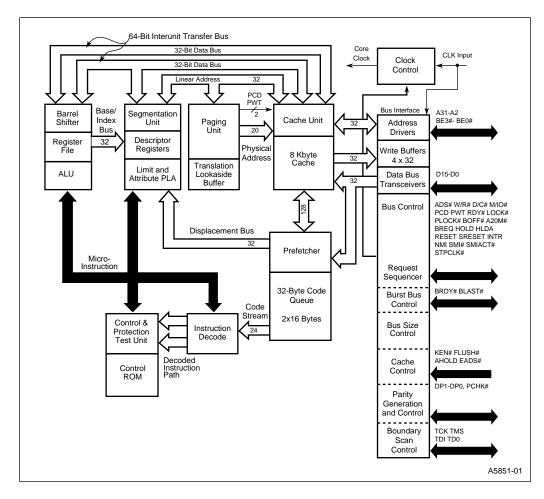
Figure 3-4. Ultra-Low Power Intel486™ GX Processor Block Diagram
