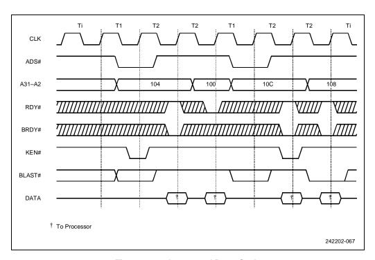
Figure 10-19. Interrupted Burst Cycle
