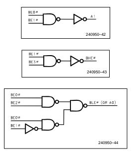
Figure 10-5. Logic to Generate A1, BHE# and BLE# for 16-Bit Buses
