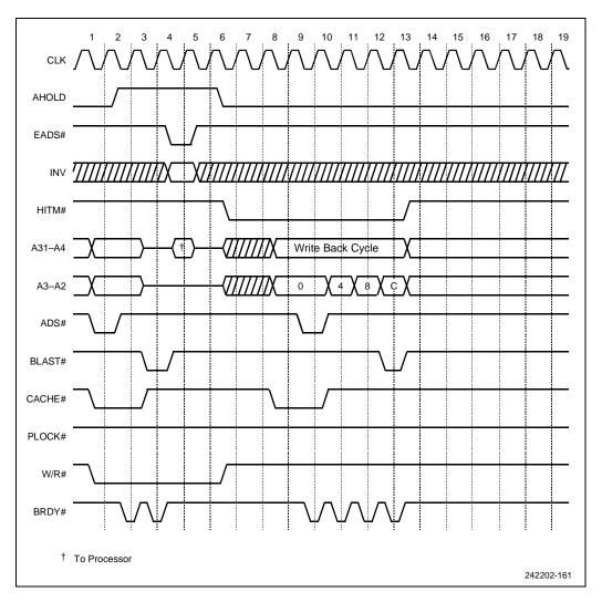
Figure 10-49. Snoop under AHOLD Overlaying Pseudo-Locked Cycle
