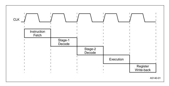
Figure 3-8. Internal Pipelining
