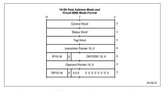
Figure 4-13. Real Mode FPU Instruction and Data Pointer Image in Memory—16-Bit Format
