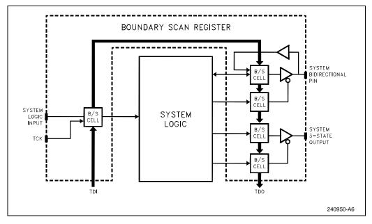
Figure B-7. Logical Structure of Boundary Scan Register
