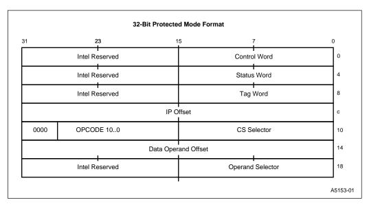
Figure 4-10. Protected Mode FPU Instructions and Data Pointer Image in Memory— 32-Bit Format
