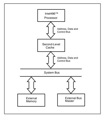
Figure 10-27. System with Second-Level Cache
