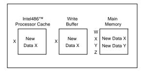
Figure 9-5. Reordering of a Reads with Write Buffers
