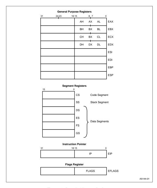
Figure 4-1. Base Architecture Registers
