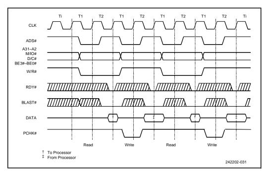
Figure 10-10. Basic 2-2 Bus Cycle
