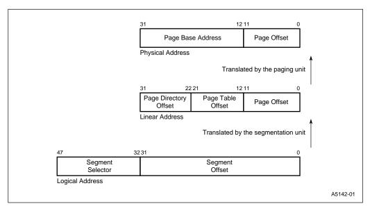
Figure 3-6. Segmentation and Paging Address Formats
