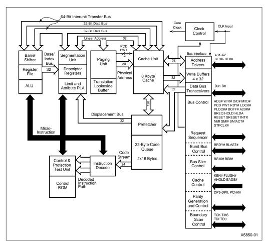
Figure 3-3. Ultra-Low Power Intel486™ SX Processor Block Diagram
