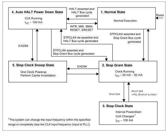
Figure 9-9. Intel486™ Processor Family Stop Clock State Machine
