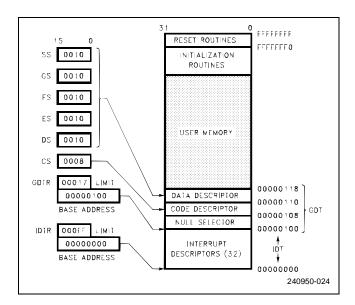
Figure 6-17. Simple Protected System
