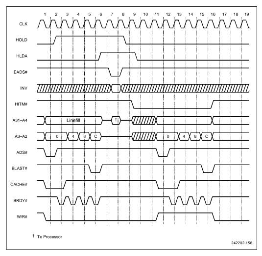
Figure 10-44. Snoop under HOLD during Line Fill
