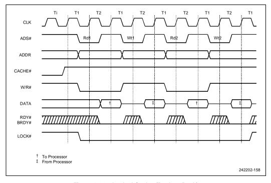
Figure 10-46. Locked Cycles (Back-to-Back)
