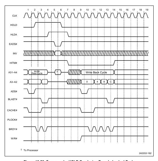
Figure 10-50. Snoop under HOLD Overlaying Pseudo-Locked Cycle
