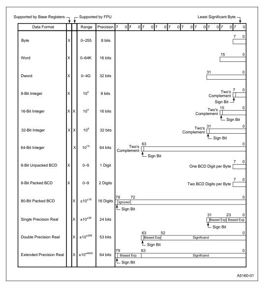
Figure 3-15. Intel486™ Processor Data Types
