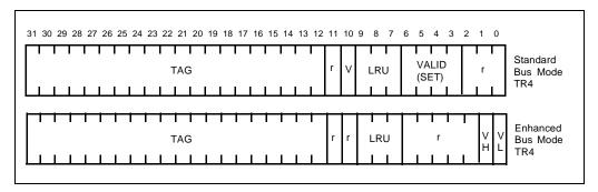
Figure B-3. TR4 Definition for Standard and Enhanced Bus Modes for the Write-Back Enhanced IntelDX4™ Processor
