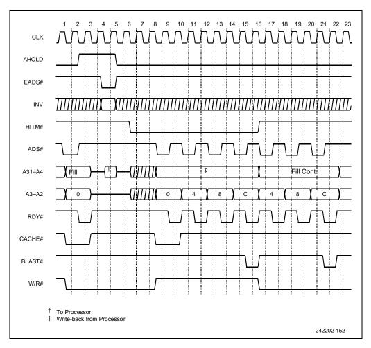
Figure 10-40. Snoop Cycle Overlaying a Non-Burst Cycle
