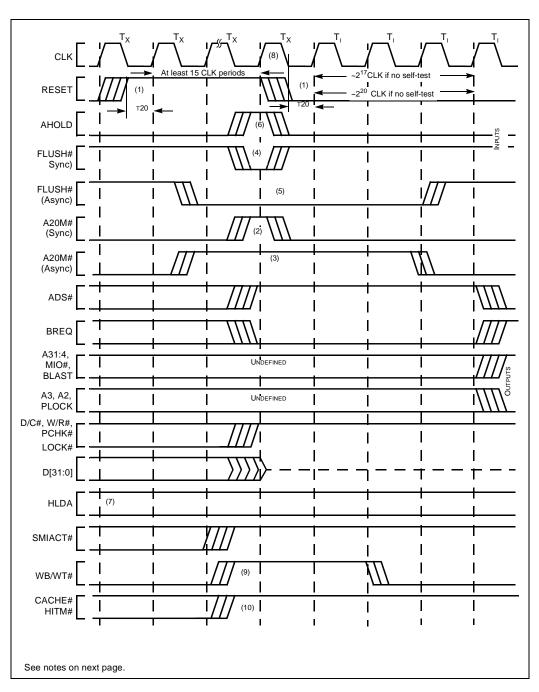
Figure 9-7. Pin States During RESET
