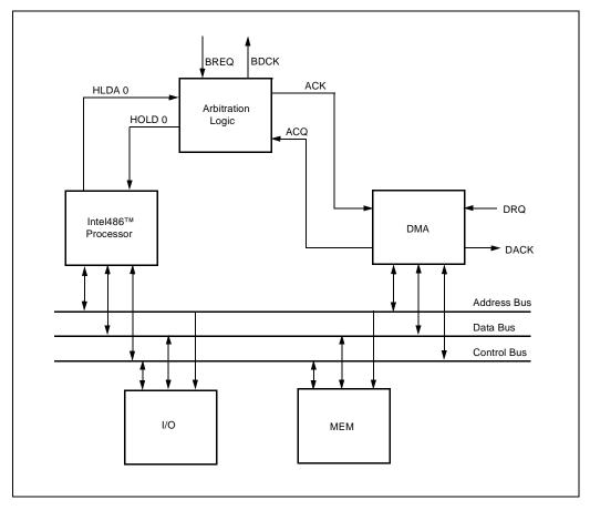
Figure 10-9. Single Intel486™ Processor with Multiple Secondary Masters
