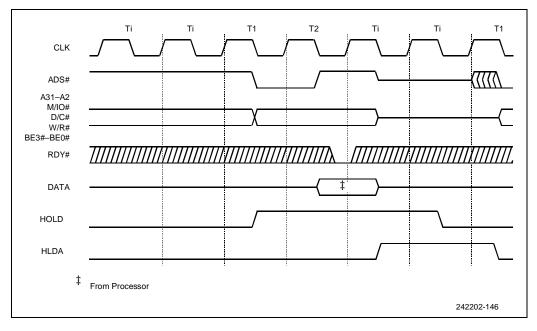
Figure 10-29. HOLD/HLDA Cycles
