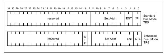
Figure B-4. TR5 Definition for Standard and Enhanced Bus Modes for the Write-Back Enhanced IntelDX4™ Processor
