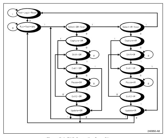
Figure B-8. TAP Controller State Diagram
