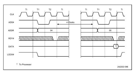
Figure 10-31. Interrupt Acknowledge Cycles
