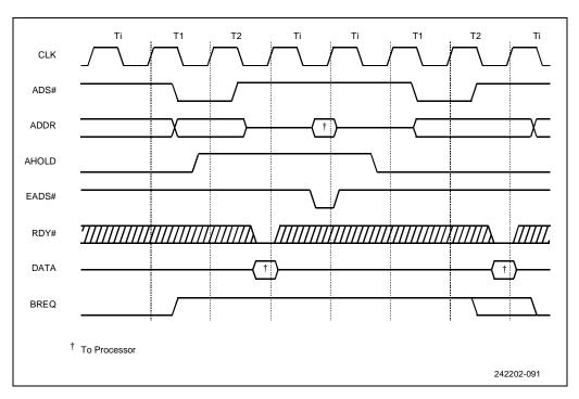
Figure 10-25. Fast Internal Cache Invalidation Cycle
