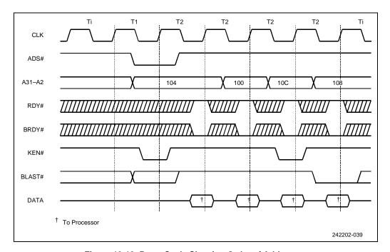
Figure 10-18. Burst Cycle Showing Order of Addresses
