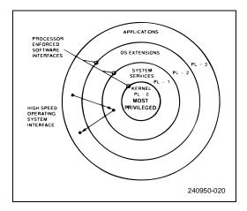
Figure 6-13. Four-Level Hierarchical Protection
